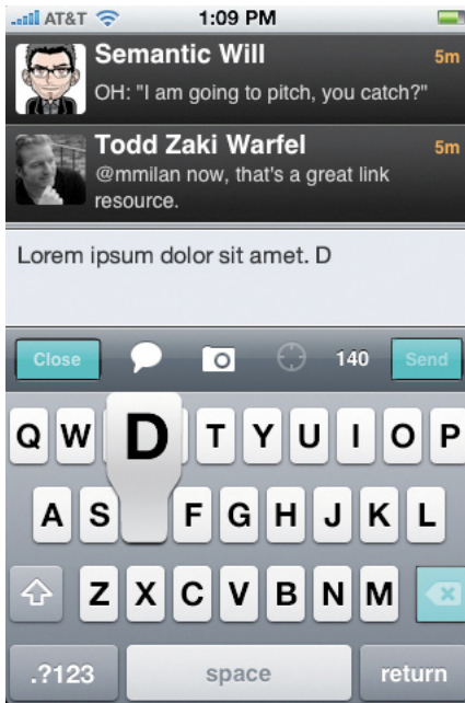
FIGURE 9.16 http://www.flickr.com/photos/rosenfeldmedia/3978898382/ Hotspots for Close, Send, and Backspace buttons on keyboard.
