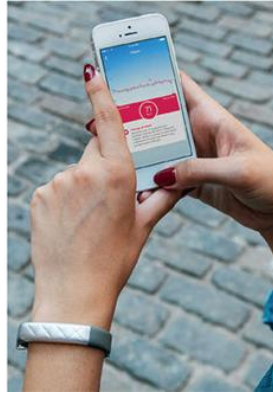
Figs 3.14 to 3.16 Worn like a wrist band, Jawbone's UP keeps track of all physical activities users do during the day, tracks sleep, and syncs with the phone via Bluetooth.
