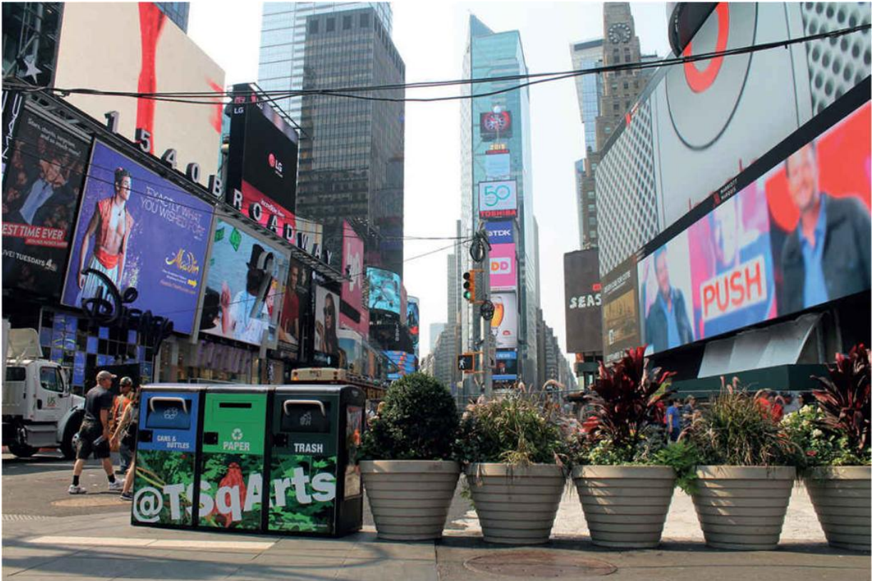
Figs 3.7 and 3.8 Bigbelly is a Smart Waste & Recycling System whose solutions include smart bins that are equipped with a sensor that measures level of waste inside, and alerts the collection system only when completely full through real-time data, reducing the need for collection by 80 percent and consequently reducing CO 2 emissions associated with trucks.
