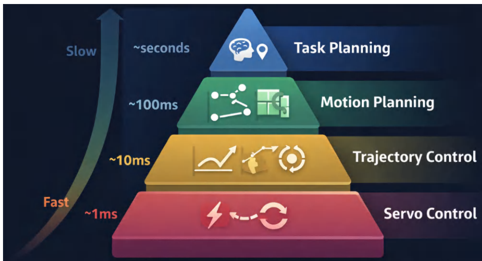
Figure 16.2 – The multi-rate control hierarchy of an Embodied Intelligence agent
